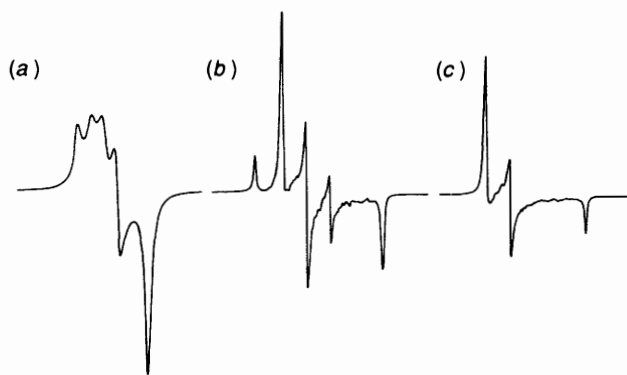
Figure 3. The e.p.r. spectra of [\text{Cu}(\text{L})\text{Cl}_2] : (a) X-band of powdery material, (b) Q-band of powdery material, (c) Q-band of crystalline material
